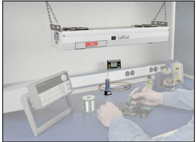
Figure 22. Using the EM Aware Monitor with ionizer antenna on a workbench with the SCS 770112 Ion Pro™ Overhead Ionizer
