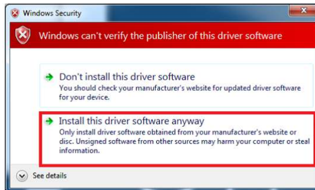
Figure 37 Confirm installation of unsigned driver
