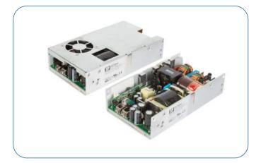
The PBR500 series of AC-DC switching power supplies, in a package of just 4 x 7 x 1.7 inches, deliver 450-500 watts of continuous power with forced air cooling or 350-400 watts with convection cooling. The units are constructed on a U-Channel for mechanical support and heat sinking. A cover and fan assembly can be added during manufacturing. They are designed for both ITE/Industrial and medical applications including those needing BF rated insulation with an operation altitude up to 5000 meters.
