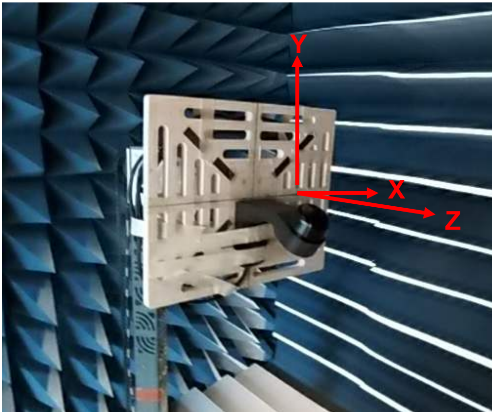
Figure.6 Testing Setup in ETS Anechoic Chamber
