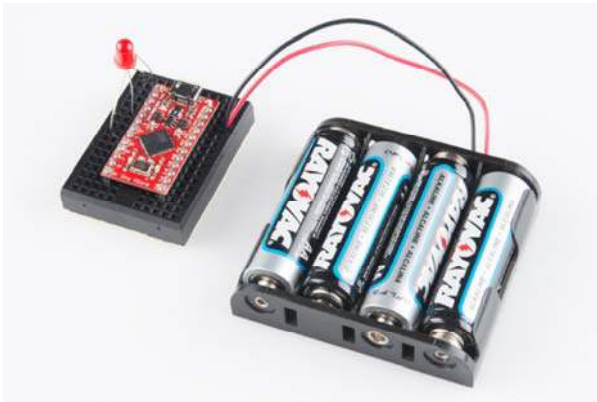
Pro Micro powered through the RAW pin by a set of four, series AA batteries.
