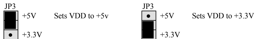
Figure 2: VDD_SEL Option Header
