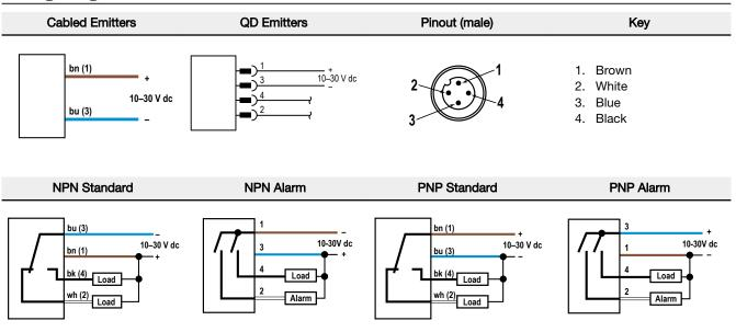
Wiring for the quick disconnect (QD) models is functionally identical.
