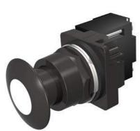
30mm BlackMax, Epoxy Coated Corrosion Resistant Complete Metal Unit Illuminated Push-Pull Operator Full Voltage, 120V AC/DC LED Lamp Mushroom Head Cap Small 1 3/4" (44.5 mm) Metal, Black with White Lens 3 Position Pull-Momentary/Push-Maintained UL Listed, CSA Certified NEMA 1,3,3R,4,4X,12,13 & Automotive Standards
