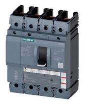
circuit breaker 3VA5 UL frame 250 breaking capacity class M 35kA @ 480 V 4-pole, line protection TM210, FTFM, In=150A overload protection Ir=150A fixed short-circuit protection Ii=10 x In N conductor protection 100% without connection
