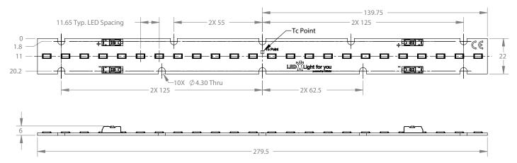
1. Four Poke-In Connectors accept 18-24 AWG solid or stranded wire
