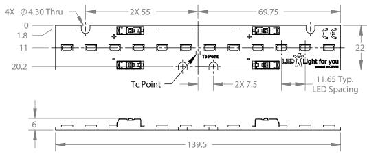
1. Four Poke-In Connectors accept 18-24 AWG solid or stranded wire
