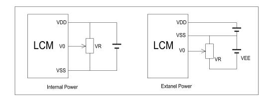
$V_{\text{DD}^{\sim}}V_{0}\text{: LCD}$  Driving voltage
