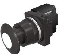
30mm BlackMax, Epoxy Coated Corrosion Resistant Complete Metal Unit Illuminated Push-Pull Operator Transformer type, 120V AC Incandescent Lamp Mushroom Head Cap Small 1 3/4" (44.5 mm) Metal, Black with White Lens 2 Position Maintained, Pull-to-Release UL Listed, CSA Certified NEMA 1,3,3R,4,4X,12,13 & Automotive Standards
