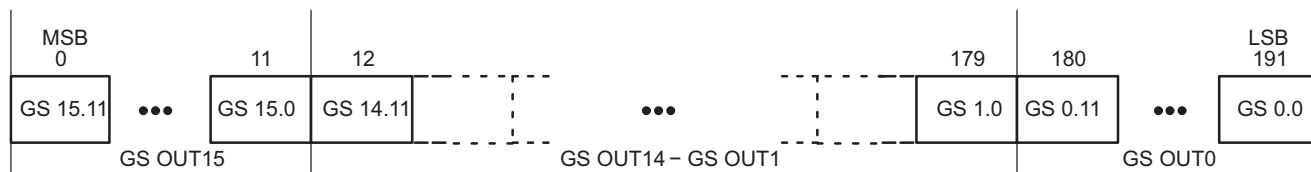
Figure 21. Grayscale Data Packet Format
