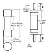
Dimension A (REF): 0.65 mm (0.5 A-6.3 A), 0.80 mm(8 A-10 A) Dimension B: For BK/packaging,  $38.1\pm0.38$  mm For TR2/ packaging,  $15.8\pm2$  mm
