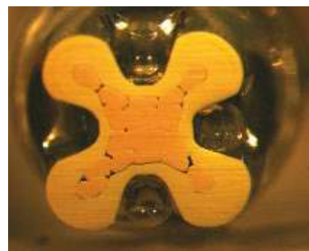
Crimp-cross section HARTING crimp profile
