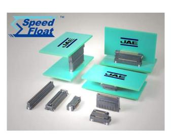
The MA01 Series is the next generation floating board-to-board connector. This product features a highly reliable two-point contact structure, achieving high-speed transmission exceeding 8Gbps. With an operation temperature range of -40°C to 125°C the connector is suitable for harsh temperature environments unique to the automotive industry.
