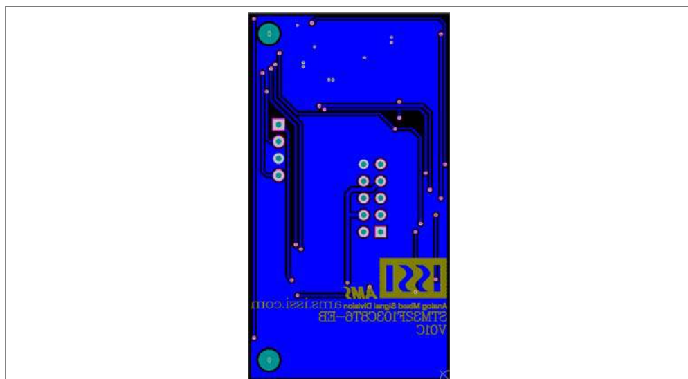
Figure 13: Board PCB Layout - Bottom Layer
