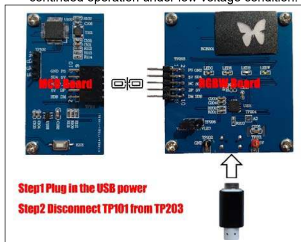
Figure 2: Photo of RGBW Board disconnected from MCU board
