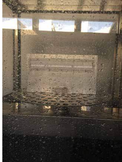
Testing under water jet
