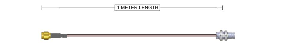
Connector A 132178 SMA Plug Straight Brass Gold + Heatshrink 50 Ohm RG-316DB Continuity/Hi-Pot Connector B 031-6332 BNC Jack Straight Bulkhead - Rear Mount Brass Nickel IP67
