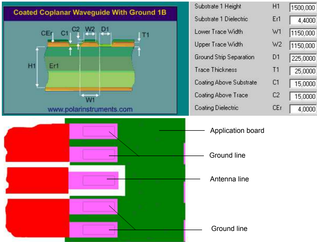
Figure 16: Micro-Stripline on 1.5mm Standard FR4 PCB - example 2
