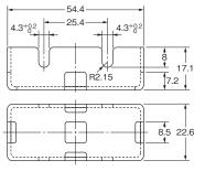
Note: The Cover has five holes for easy lead wire connections.
