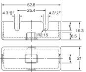
Note: The Cover has five thin, easy-to-separate portions for easy lead wire connections.
