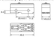
Note: 1. Appropriate terminal screw tightening torque: 0.78 to 1.18 N·m.
