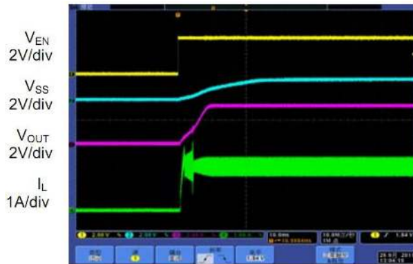
Fig. 12: Enable turn on ( R_{LOAD}=1.65\Omega ) Base Time 10ms/div
