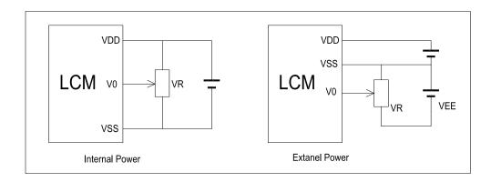
$V_{DD^{\sim}}V_0\text{: LCD Driving voltage}$
