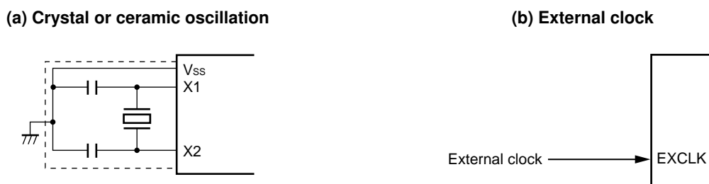
Figure 5-9. Example of External Circuit of X1 Oscillator
