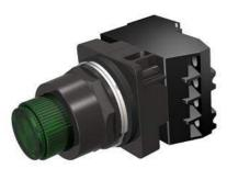
30mm BlackMax, Epoxy Coated Corrosion Resistant Complete Metal Unit PTT / Illuminated Pushbutton Full Voltage, 6V AC LED Lamp Extended Button Plastic Lens, Green 2 Position Momentary with 1 N.O. - 1 N.C. Heavy Duty Contacts, A600/P600 UL Listed, CSA Certified NEMA 1,3,3R,4,4X,12,13 & Automotive Standards
