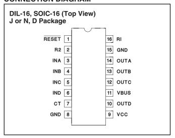
**ELECTRICAL CHARACTERISTICS:** Unless otherwise stated these specifications <u>apply for T<sub>A</sub> = -55°C to +125°C for UC1702; -25°C to +85°C for UC2702; 0°C to +70°C for UC3702; VBUS = 34V, VCC = 5V, RESET = VCC, R2 = 43.2kΩ; R1 = 203kΩ; CT = 220pF, T<sub>A</sub> = T<sub>J</sub>.</u>
