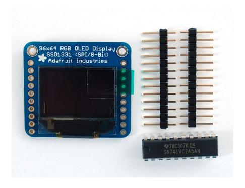
Since the OLED is 3.3V and also uses 3.3V logic, we need to use a logic shifter. We include a DIP logic shifter, the 74LVX245 with the OLED. If you're using a 3.3V logic
