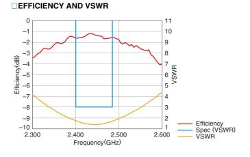
• Tested antenna has been soldered. Evaluation board size is 50x20x1 mm.
