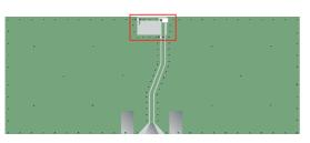
PCB size : 50mm x 20mm x 1mm Antenna area : 5 x 3 mm
