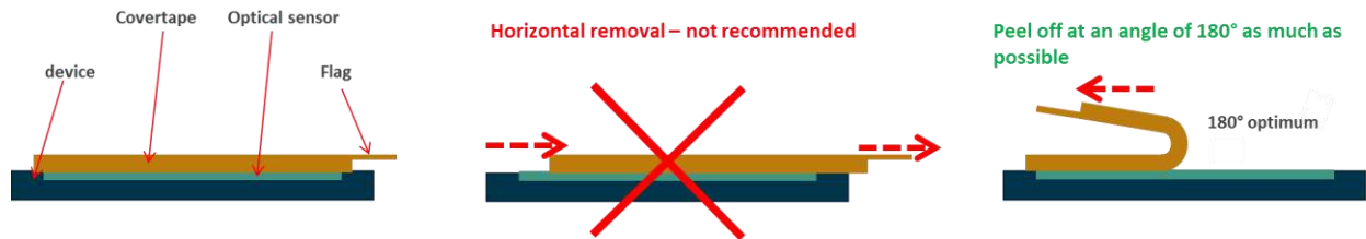
Figure 33: Grab the flag of the covertape and peel it off in an angle of 180° as much as possible.
