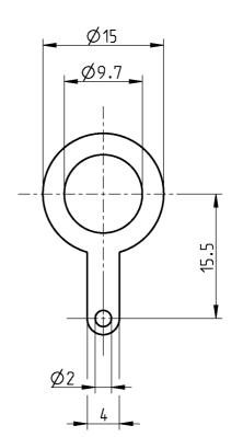
All dimensions are in mm; tolerances according to ISO 2768 m-H
