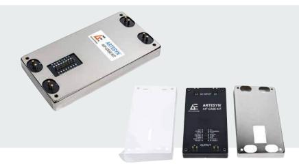
The AIF case kit is for AIF series of high voltage DC-DC converters which comprises six single output models offering voltages of 1.8 V, 3.3 V, 5.0 V, 12 V, 15 V or 24 V. Designed for use with power factor correction (PFC) modules, the converters accept a wide range input of 250 to 420 Vdc.
