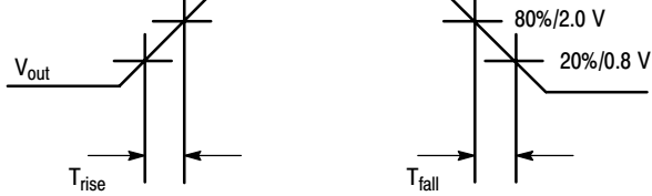
Figure 14. Waveforms: Rise and Fall Times
