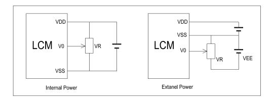
$V_{DD\sim}V_0$ : LCD Driving voltage VR:  $10k\sim20k$
