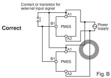
The PM5S series is provided with a transformerless power supply.
