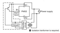
• Input and Power supply circuit
