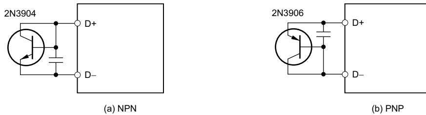
Figure 88. Remote Temperature Sensor Using Transistor
