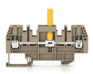
Test disconnect terminal, Screw connection, Mounting type: Mounting rail TS 35/7.5, Rated cross-section: 6 mm², Width: 8.1 mm, Colour: Beige
