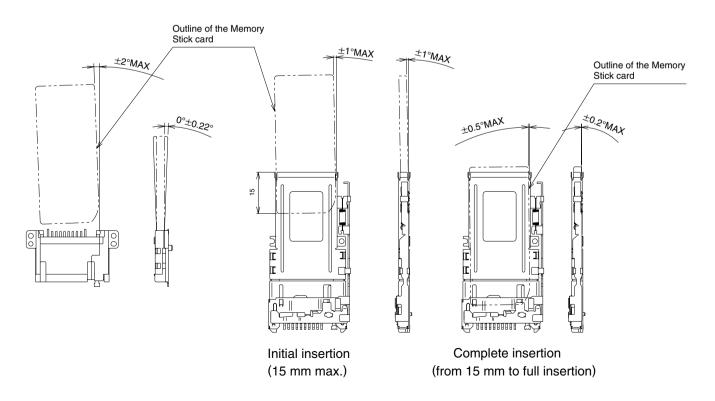
3.When inserting or withdrawing cards from the CB1C Series, the side contacts on both sides will protrude outward by 0.6 mm. Care should be taken that they will not be restricted or touch other components.
