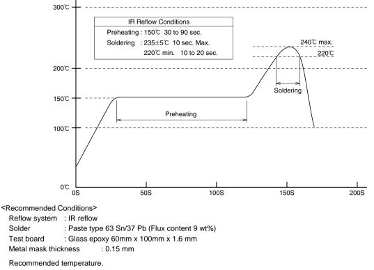
The temperature may be slightly changed according to the solder paste type and volume used.
