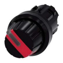
Selector switch, illuminable, 22 mm, round, plastic, red, Rotary knob, 2 switch positions O-I, latching, actuating angle 90°, 10:30h/13:30h, with laser labeling, inscription or symbol Customer-specific selection with SIRIUS ACT configurator (CIN)
