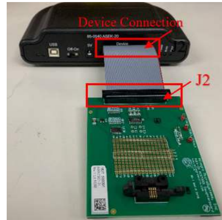
Figure 8: Connection between ASEK-20 and ASEK70310 Daughterboard
