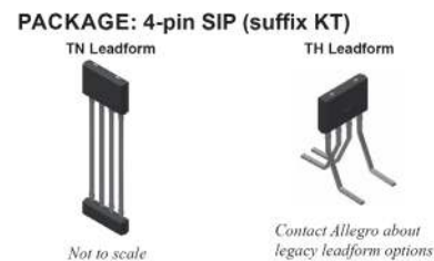
Figure 9: KT Lead-forming Options
