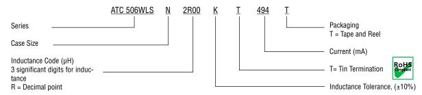
The above part number refers to a 506WLS Series, Case Size N, 2.00  $\mu$ H inductor, K tolerance (±10%, typ.), with Tin Termination (T), 494 mA, tape and reel packaging..
