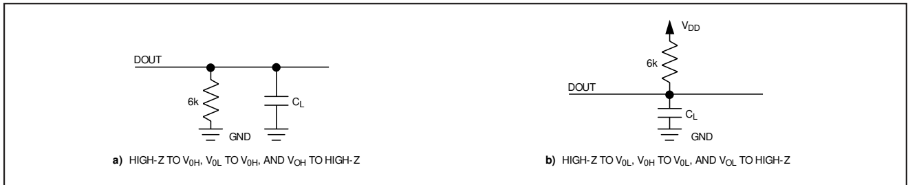
Figure 1. Load Circuits for Enable and Disable Time
