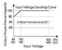
With an AC input between 85-100VAC and a DC input between 120-140VDC, the output power must be derated as per temperature derating curves;
