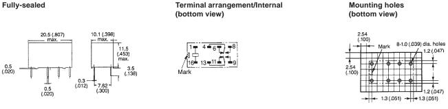
Note: 1. ####and [\_\_] indicate mounting orientation marks. 2. A tolerance of  $\pm 0.10$  (0.004) applies to the above dimensions.
