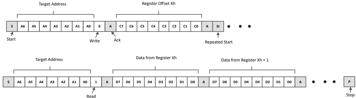
Figure 8-13. I2C Read with Repeated Start
