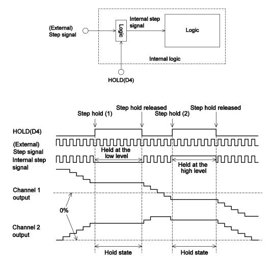
When the hold bit in the serial data, D4 (100, \*, D4, \*\*\*), is set to 1, the external step state at that time is held without change as the internal step state.
