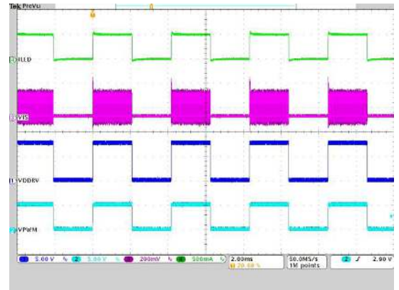
Ch1: DDRV voltage; Ch2: PWM input; Ch3: Switch sense current resistor voltage; Ch4: LED current; Time: 2 ms/div Figure 38. PWM Dimming Transient
