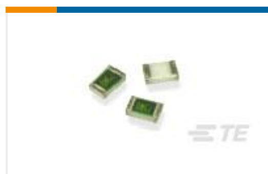
TE Part #6-2176093-6 RP 2A 0.25W 49K9 0.1% 25PPM 1K RL
