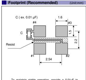
To maintain stable operation, provide a 0.01uF to 0.1uF by-pass capacitor at a location as near as possible to the power source terminal of the crystal product (between Vcc - GND).
