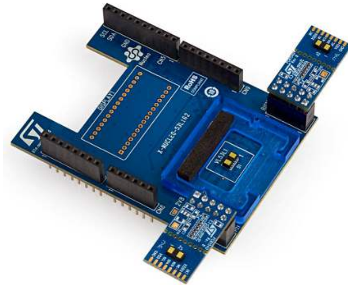
Figure 2. Connections of VL53L1 breakout boards
