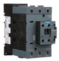
Electrically held lighting contactor, Contactor amp rating 100A, 0 N.C. / 3 N.O. Poles, 480VAC 60HZ coil, 1 NO / 1 NC auxiliary contacts Non-combination type, (no disconnect device), Enclosure NEMA type (open), No enclosure
